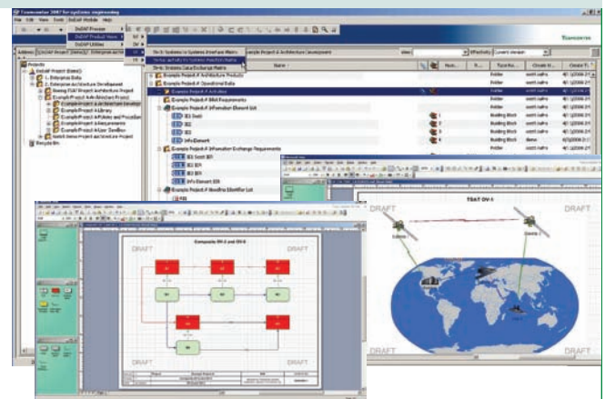
Teamcenter Systems Engineering's Explorer-like client user interface along with living DoDAF OV-1 and SV-3 diagrams.
